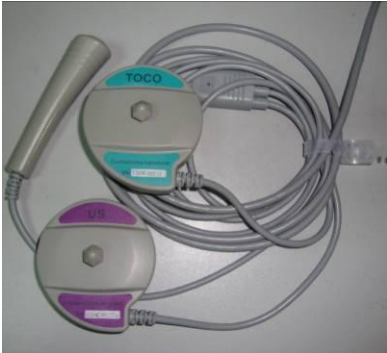
Three-in-one probe FHR probe Uterine contraction pressure probe Fetal movement mark button
