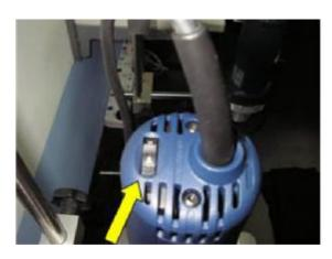
The speed is selected by the control knob on the top of the drive. Approximate rpm of the drive is:
