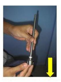
Remove totor stator and teflon bearing
