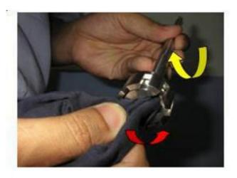
Next hold The rotor with the cloth and turn the axle clockwise(yellow arrow) or hold the axle and turn the rotor anticlock wise(red arrow)
