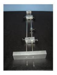
Once this bottom "H" has been fixed, take the dou ble rod and insert into the middle piece of the foo t stand. Turn it around and fix it with the other allen key using the smaller screws for it. Turn it a round and fix the drive with the support rod at the upper bosshead and the strap clamp at the lower bosshead.
